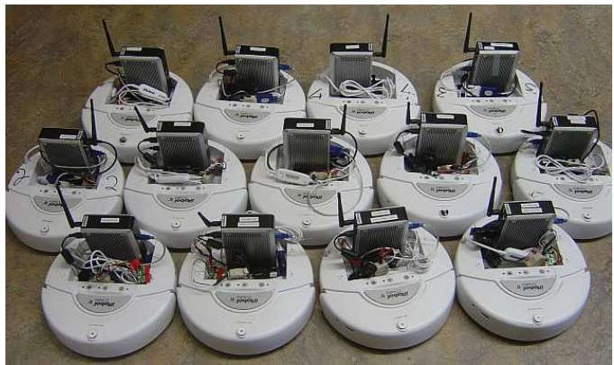
Fig. 2. This picture shows a team of iRobot Creates with an Ebox, the platform used for experiments in this work.
